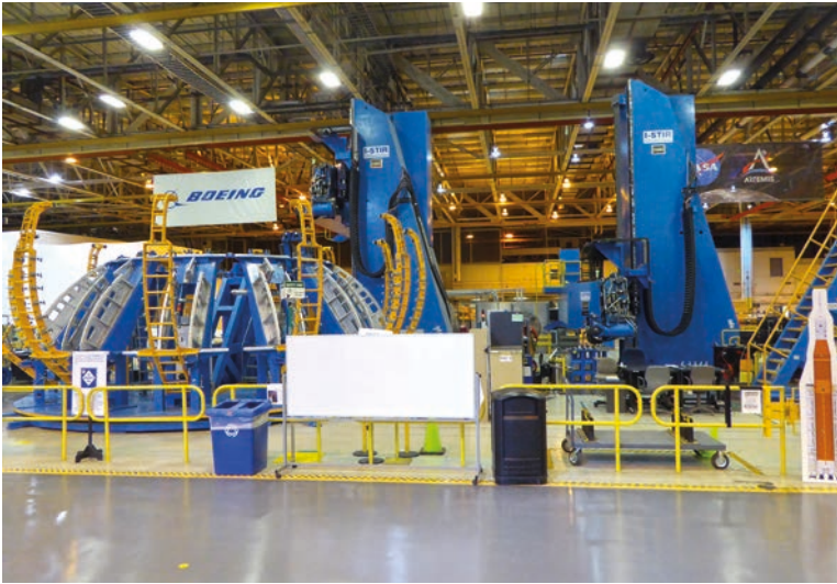
ABOVE Developed for the Shuttle External Tank, the Friction Stir Welding technique has been crucial for assembly of the core stage barrel segments.
